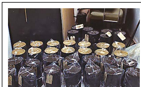
Figure 5-16: CLSM compression test cylinders. Note the color difference between those CLSMs based on Class F (dark) and Class C (light).
