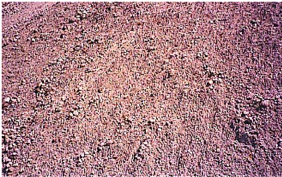
Figure 6-10: Recovered coal ash from the Pleasant Prairie Power Plant ash landfill
