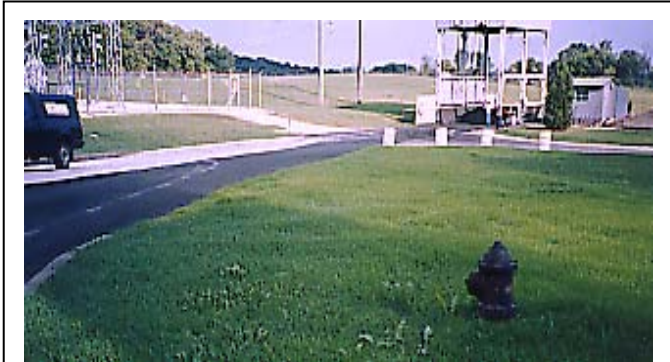
Figure 6-6: "After" grass is growing on landscaping with Scott's Hyponex 10% bottom ash topsoil blend at We Energies' Milwaukee County Power Plant.
